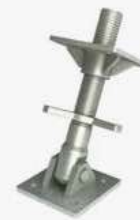
Adjustable Pivot End Compression = 210kN* Tension = 85kN *prop length at 3m
